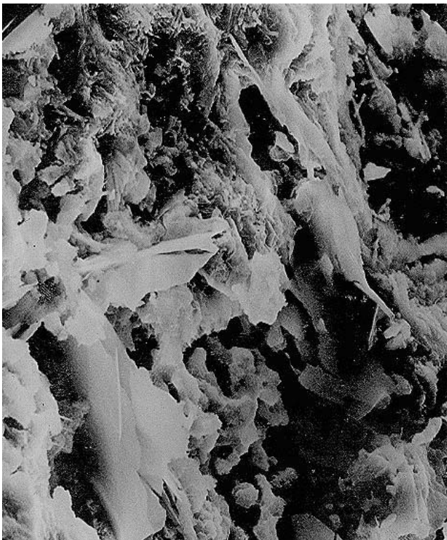
Slika 1. Mikrostruktura betona, \times 100 Figure 1. Microstructure of concrete, \times 100 .
