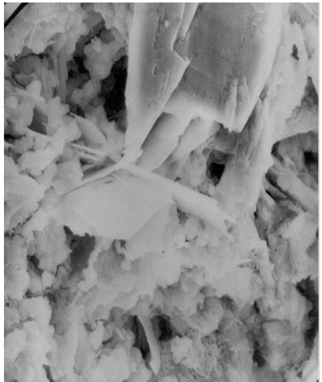
Slika 1. Mikrostruktura betona, \times 1000 Figure 1. Microstructure of concrete, \times 1000 .
